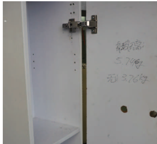
Pic. 2: Hinge mounted with a door (1)
