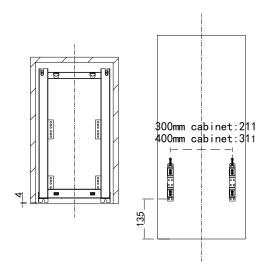
2. Adjust panel's position and fix it with screwas shown.
